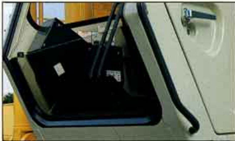
• Crossbar eliminated for wide forward visibility
