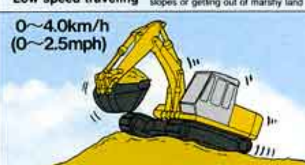
Low speed traveling traveling on site, climbing up steep slopes or getting out of marshy land
