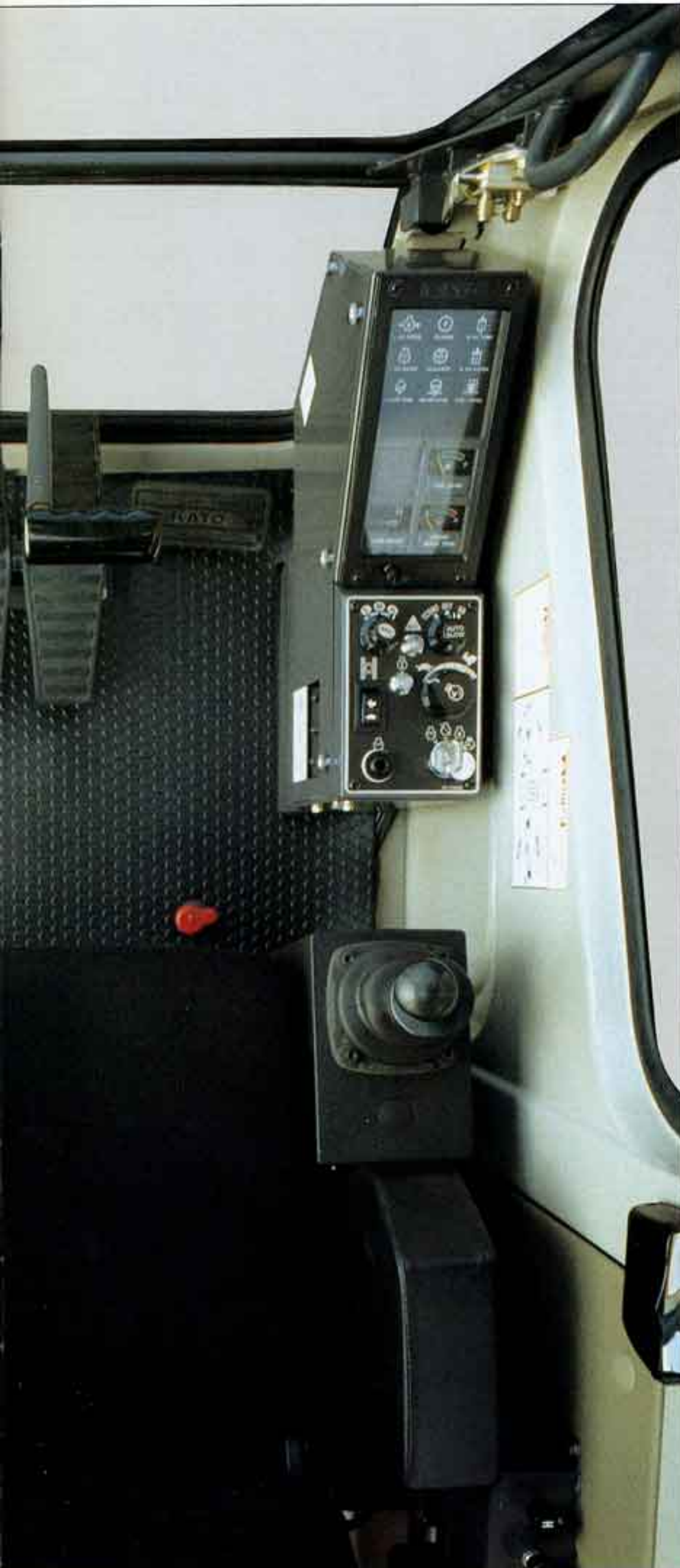
• King-size cab meets ISO international standard (940 mm)
