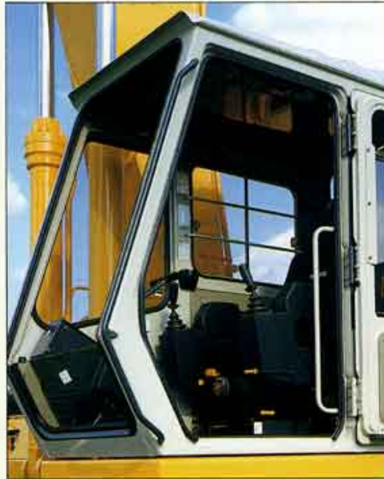
• King-size cab meets ISO international standard (940 mm)
