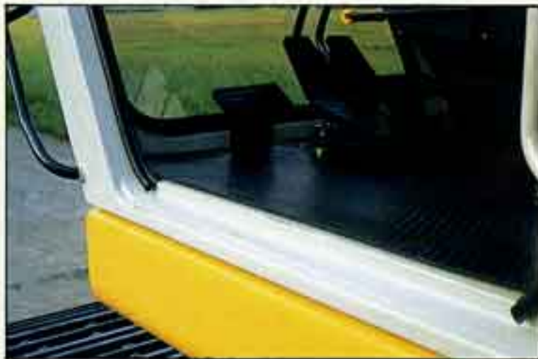
• Flat floor making access and cleaning easy
