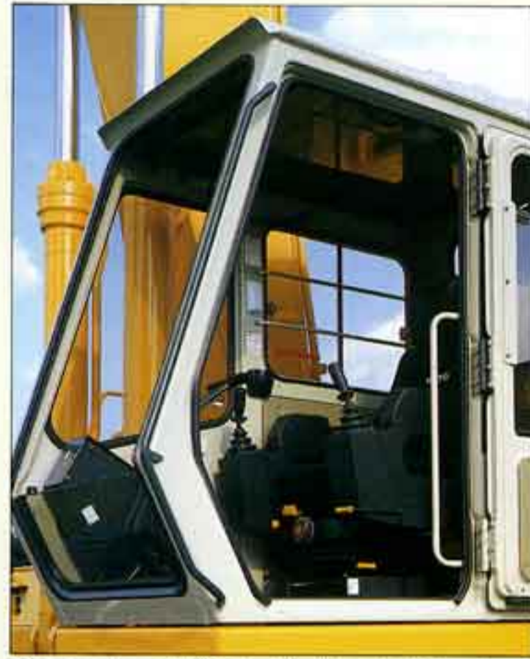
• King-size cab meets ISO international standard (940 mm)
