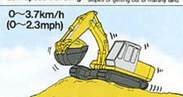
Low speed traveling traveling on site, climbing up steep slopes or getting out of marshy land
