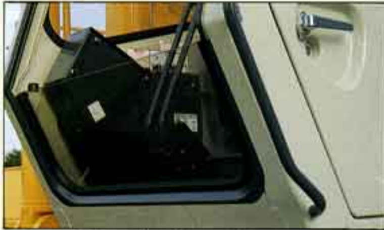
• Crossbar eliminated for wide forward visibility
