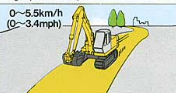
Low speed traveling traveling on site, climbing up steep slopes or getting out of marshy land
