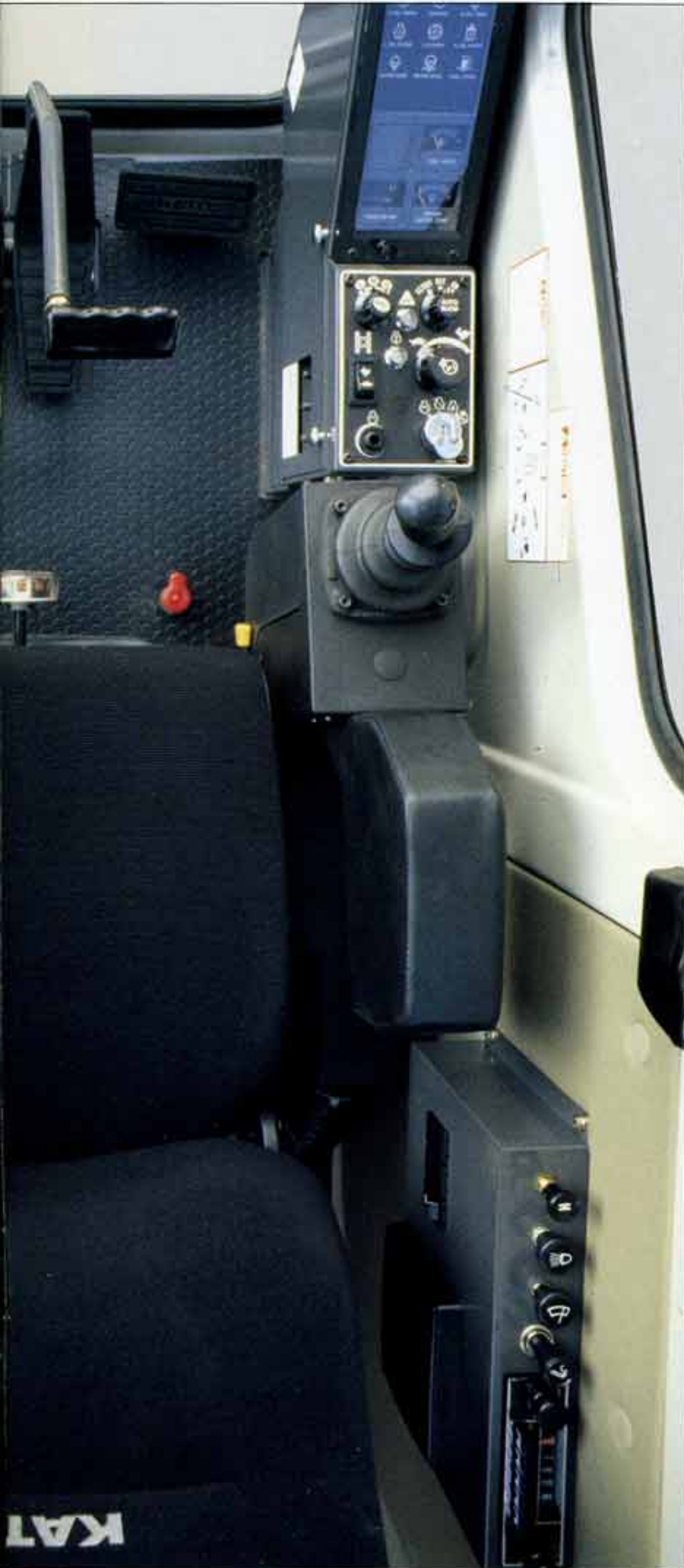
• King-size cab meets ISO international standard (940 mm)
