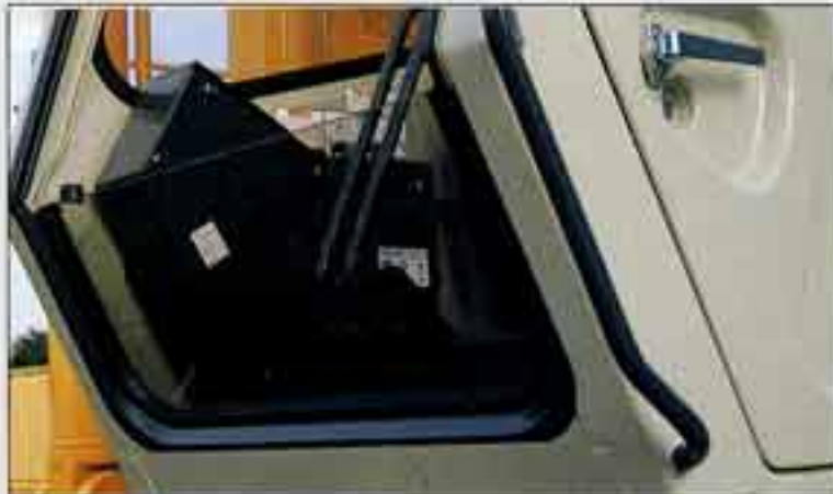
• Crossbar eliminated for wide forward visibility
