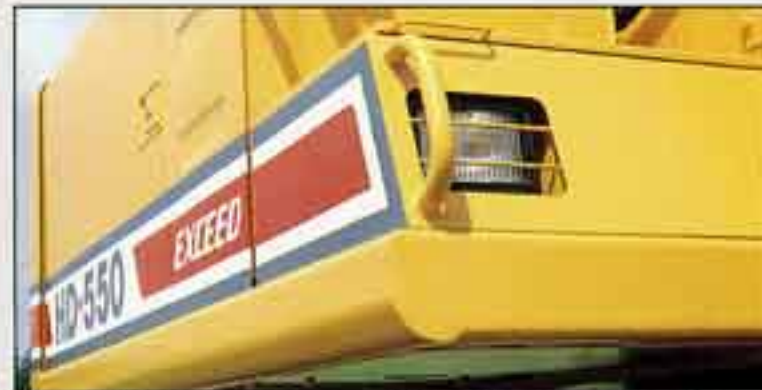
• Sturdy frame-structure prevents the engine cover from the damage
