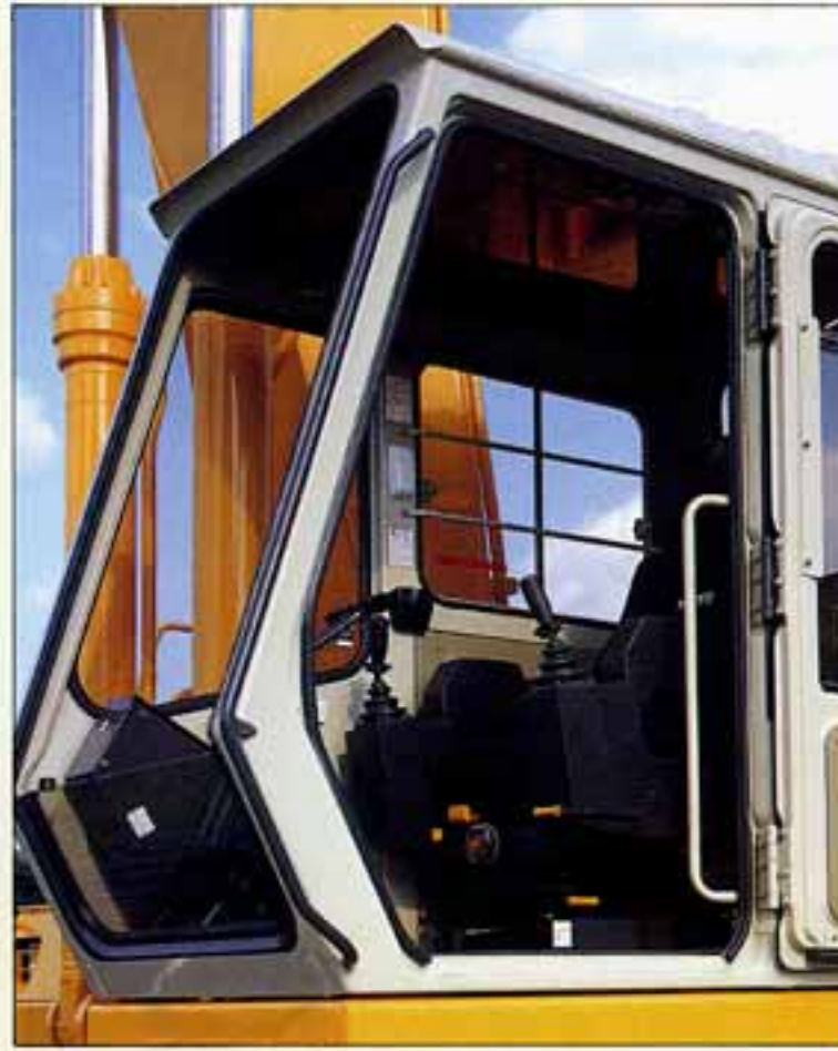
• King-size cab meets ISO international standard (940 mm)
