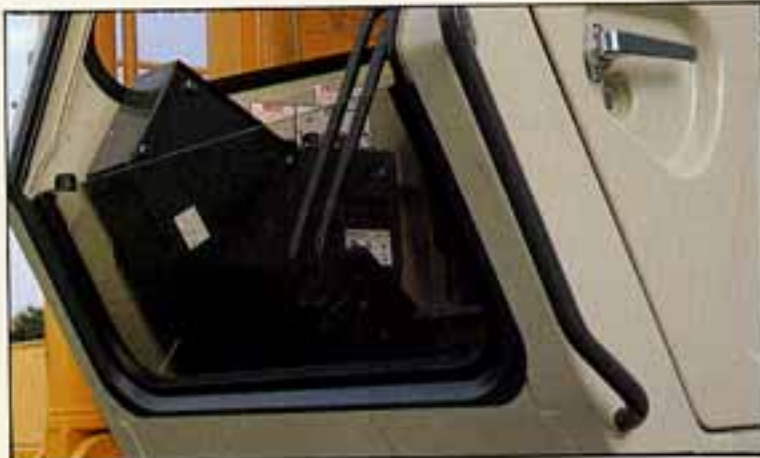
• Crossbar eliminated for wide forward visibility
