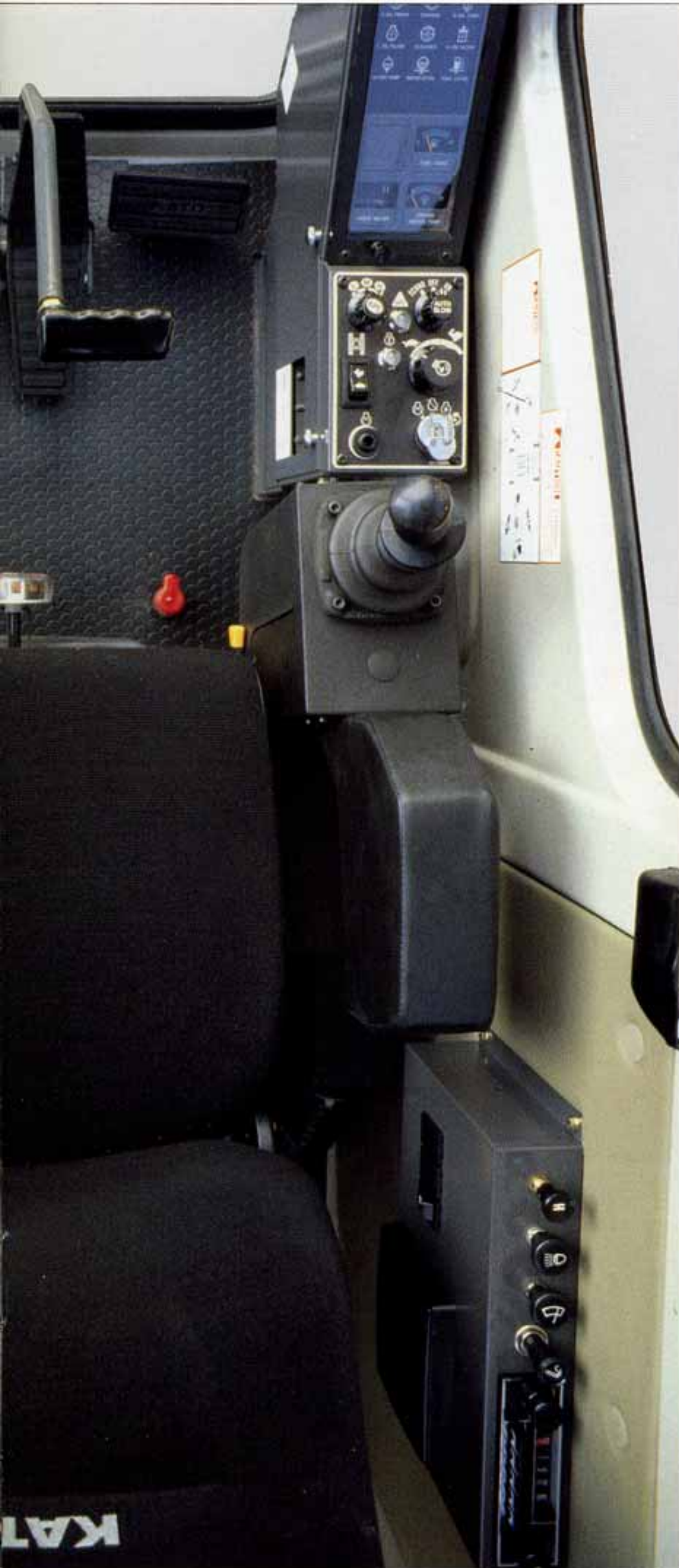
• King-size cab meets ISO international standard (940 mm)
