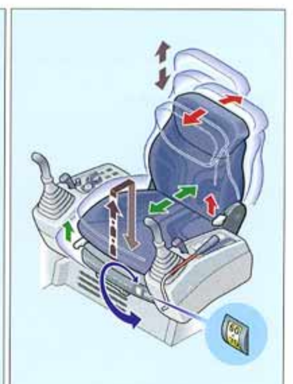
● Multi position operator's seat and adjustable seat suspension.
