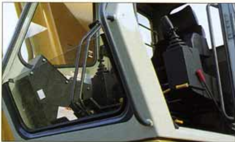
• Crossbar eliminated for wide forward visibility
