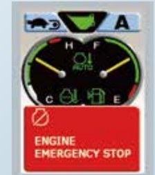
◀ When engine emergency stop switch is operated
