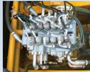
▲ Including new control valve, increased the diameter of hydraulic piping diameter
