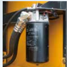
▲ Engine oil filter configuration is more efficient The filter can be replaced without go through under the body with better maintainability and safety.
