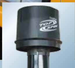
▲ New air pre-filter that does not require the special maintenance
