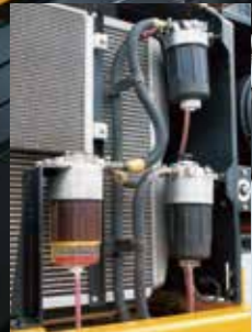
▲ Fuel filter By arranging the triple filters in the same position to improve the efficiency of replacement. Easy to access and improve safety.
