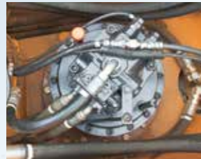
▲ Easier maintenance of swing motor ● Filling port with extension pipe ● Drain pipe diameter increase ● Top surface remote lubrication grease port
