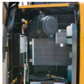
▲ Parallel configuration oil cooler and radiator
