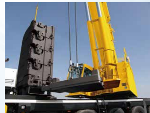
▲ Example of counterweight assembly (detaching side base)
