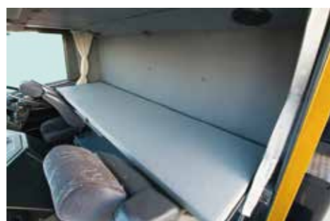
▲ large size retractable bed (2320mm×600mm)
