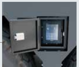
▲Outrigger touch screen control panel
